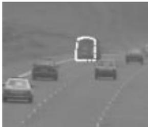
Figure 7: Tracking trucks: the affine variability allows the tracker to adjust for larger vehicles
